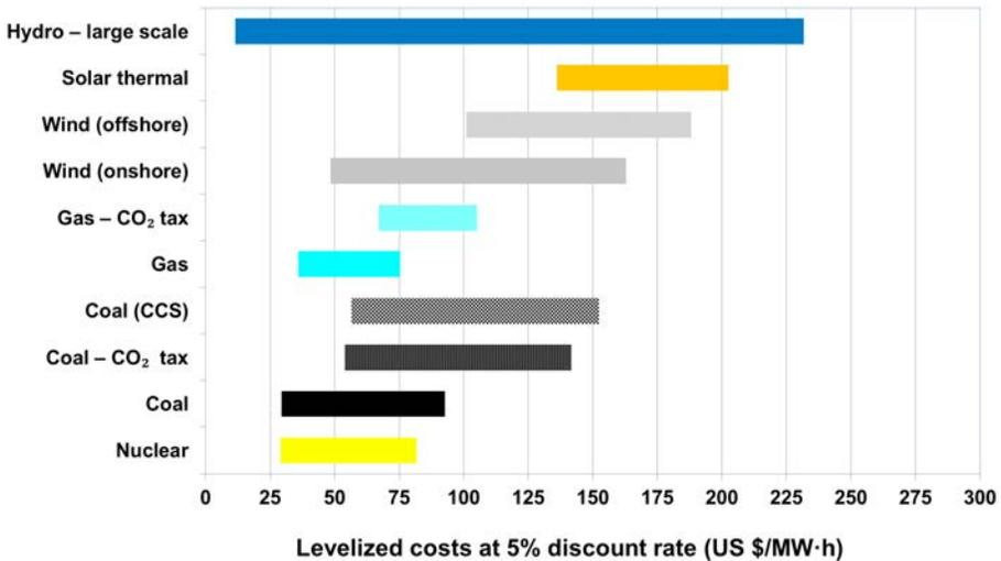
FIG. 20. Ranges of LCOE associated with new construction at 5% discount rate. Data source: Ref. [66].
