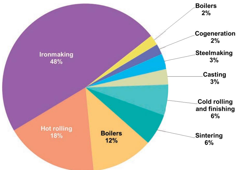
FIG. 13. Breakdown of energy consumption in iron and steel production. Source: Ref. [33].
