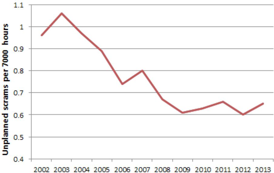
FIG. 28. Total number of unplanned scrams, including both automatic and manual scrams per 7000 h of critical power reactor operation. Data source: Ref. [103].
