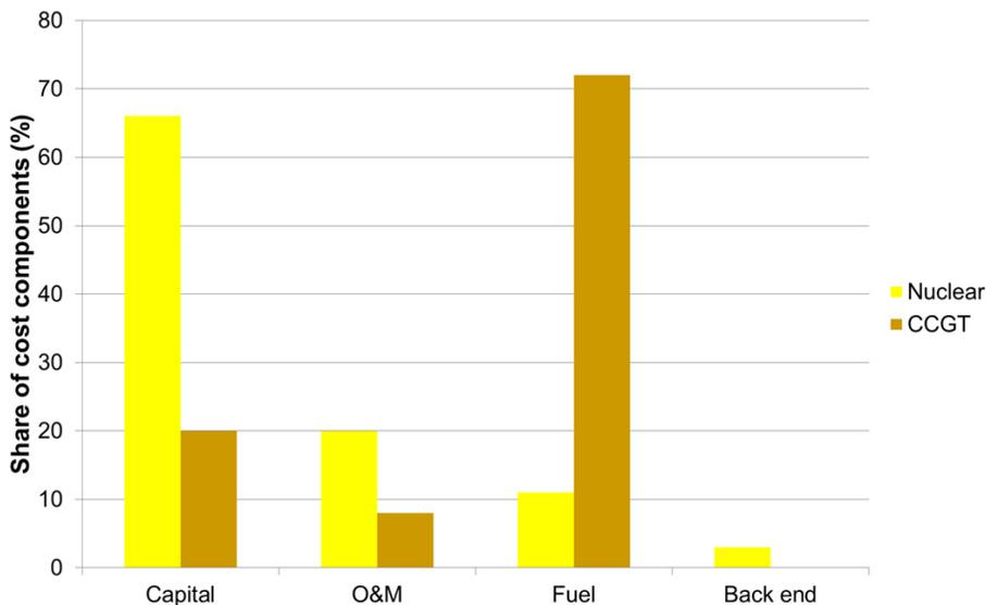
FIG. 23. Cost profile of nuclear versus gas fired generation. Note: O&M — operation and maintenance, CCGT — combined cycle gas turbine. Data source: Department of Trade and Industry [78].
