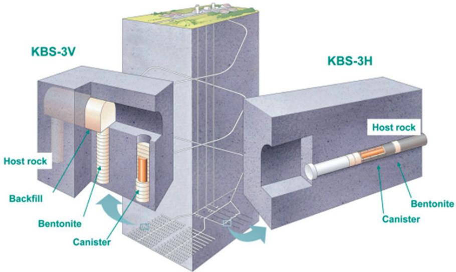
FIG. 29. The KBS-3 disposal concept. (Sources: Refs [122, 123]) (Note: KBS — nuclear fuel safety; H — horizontal; V — vertical.)
