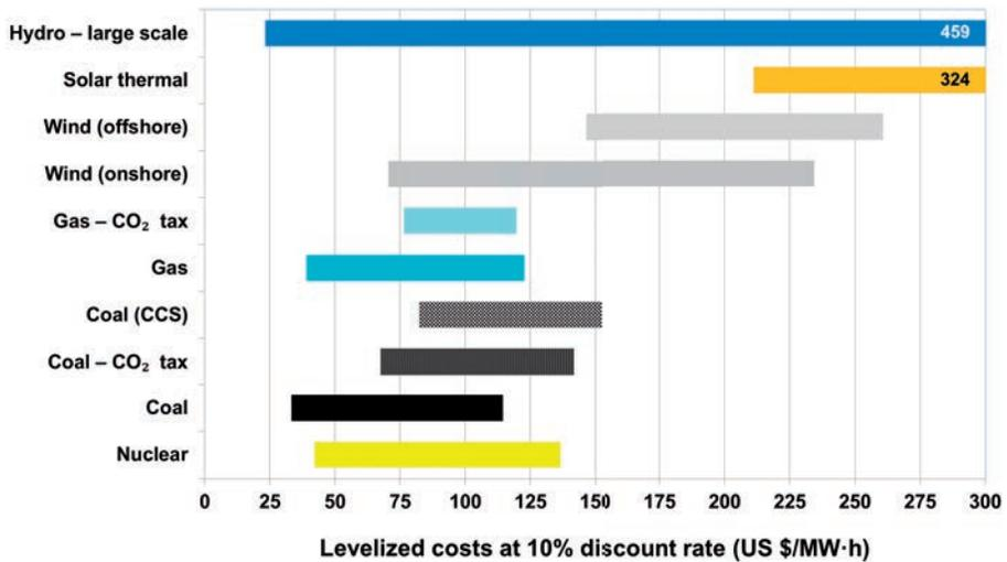
FIG. 21. Ranges of LCOE associated with new construction at 10% discount rate. Data source: Ref. [66].
