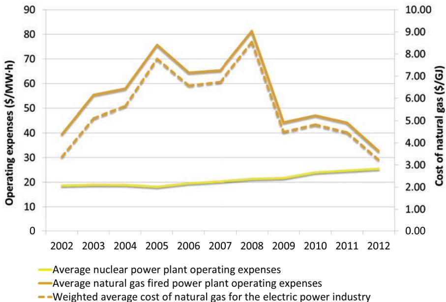
FIG. 35. Average power plant operating expenses for an average nuclear and natural gas fired power plant in the USA (left axis) compared with average cost of natural gas for the power industry (right axis). Data source: Ref. [147].
