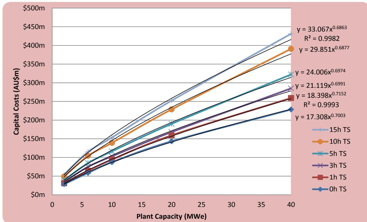
The costs include a backup boiler with 25% full-load capacity in all cases, giving quick start-up capabilities to allow the compensation of DNI fluctuations when TES is empty (Peterseim et al. 2012). Plants smaller than 20MW<sub>e</sub> are modelled without steam reheating, while larger units include single steam reheating.<sup>5</sup>
