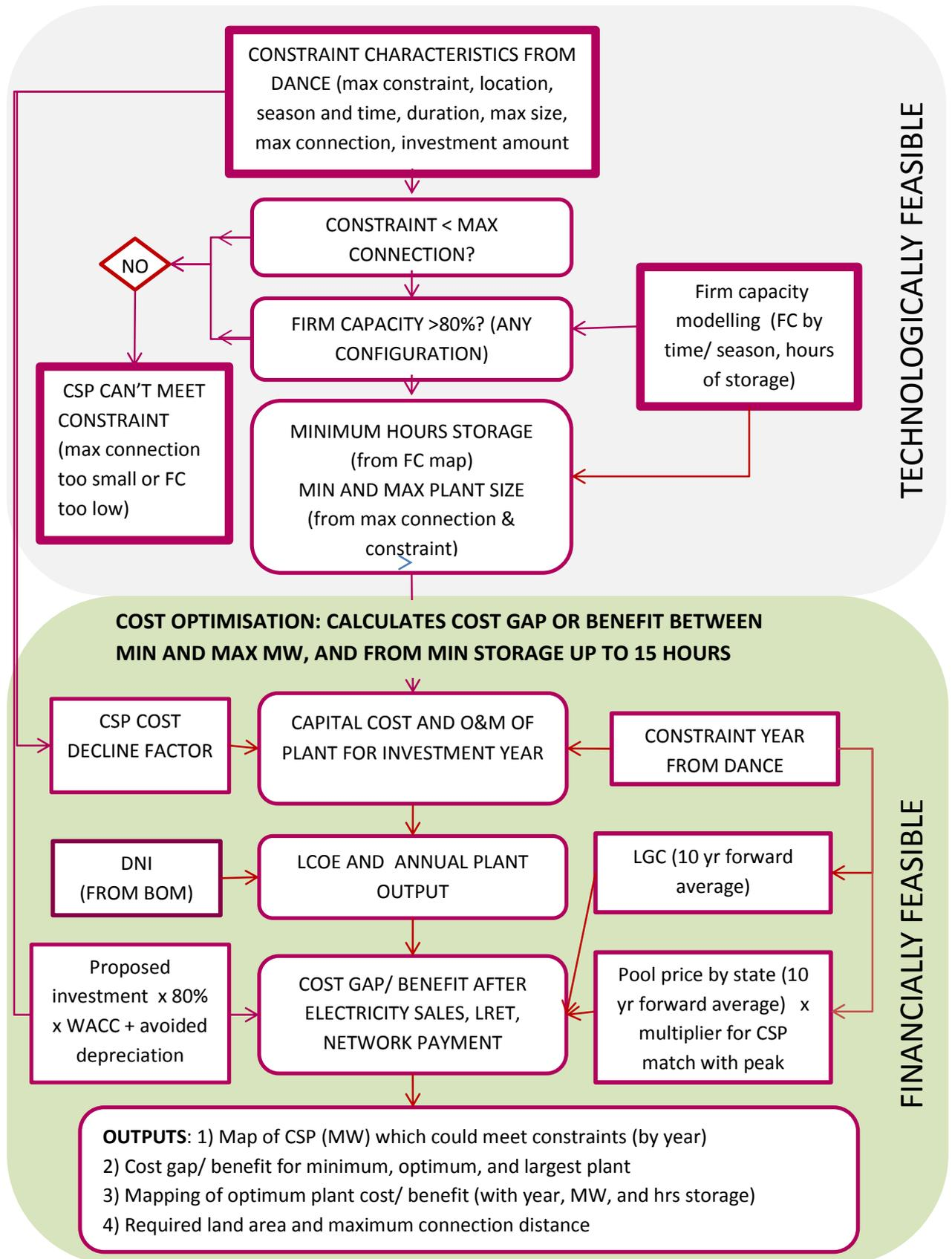
The minimum hours of storage capacity for the plant is determined by the IFC mapping, and is taken as the least hours of storage required for the plant to achieve 80% IFC at the relevant network constraint location, time of day, and season.
