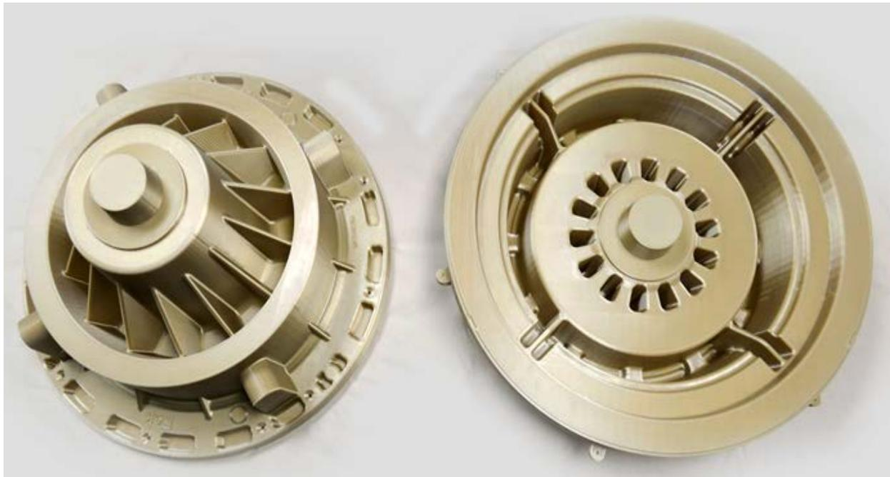
**Figure 20. Aluminum gearbox parts produced using 3D-printed sand casts (Shoemaker 2017)
