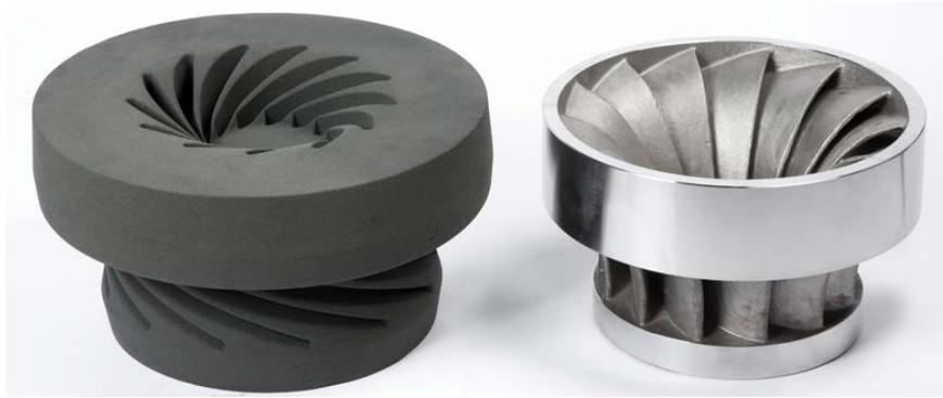
**Figure 21. Sand cast made via AM [left] and the resulting runner [right, (Voxeljet AG 2015)]
