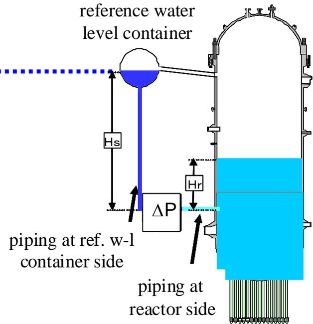
After correction, values of measured water level agree with maximum water level. Actual water level may be higher than that. Therefore, Two phase fluid will flow into RCIC turbine.
