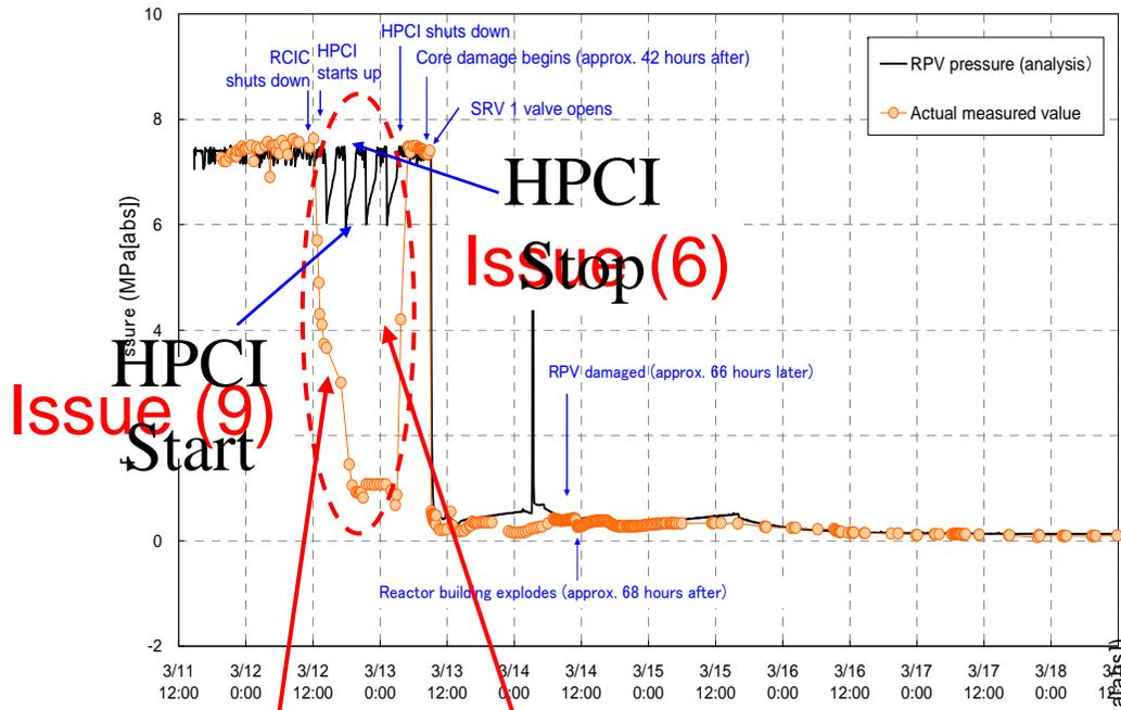
Calculated value of RPV pressure does NOT agree with measurement.
