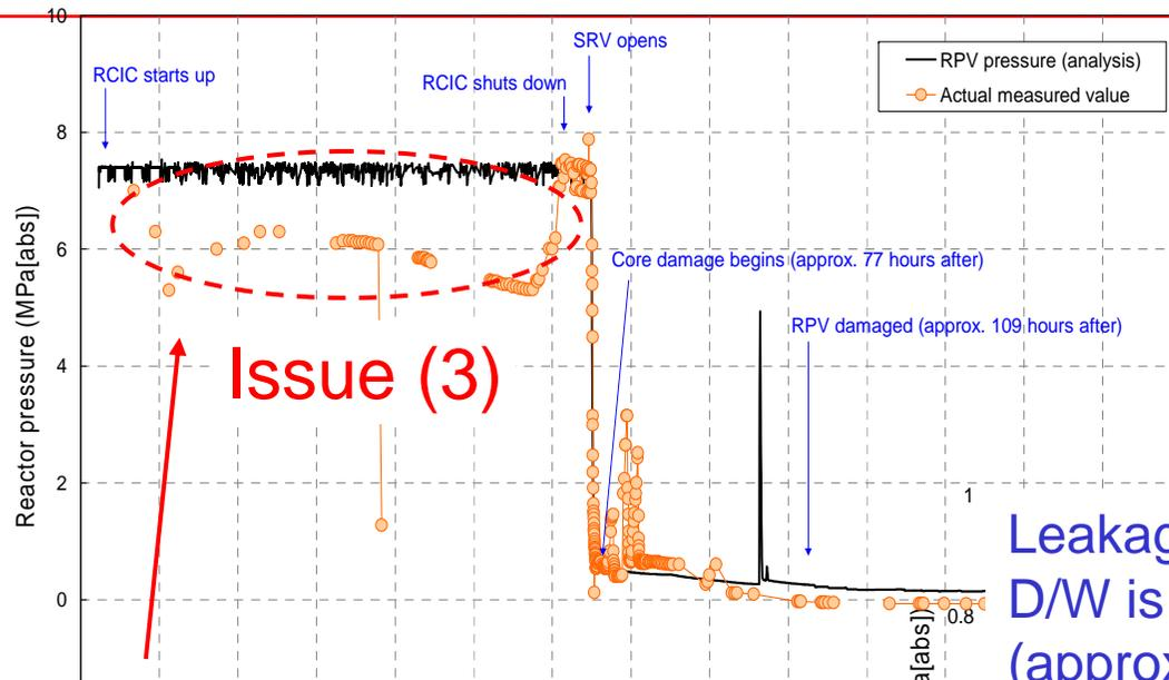
By employing assumption of gas leakage from PCV, Calculated value of PCV pressure decrease quickly, but measurement keep high pressure until morning on 3/15.
