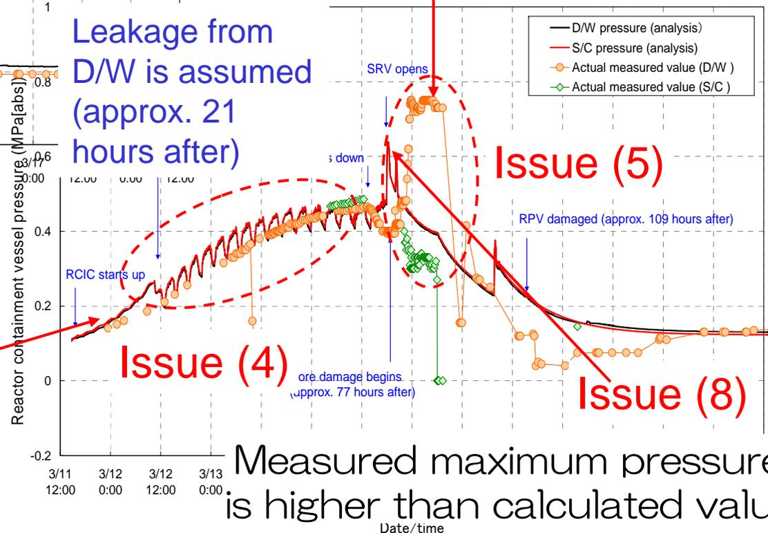
Measured maximum pressure is higher than calculated value.
